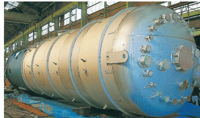
堅型円筒形整粒槽 (一圧) [3,550 φ ×16,750 H ] (SUS)
