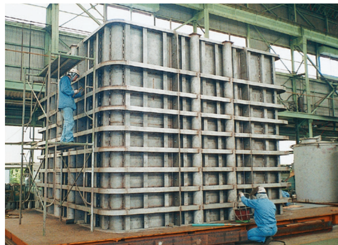
沈殿槽 [4,900 L ×4,900 W ×4,200 H ] (SUS)
