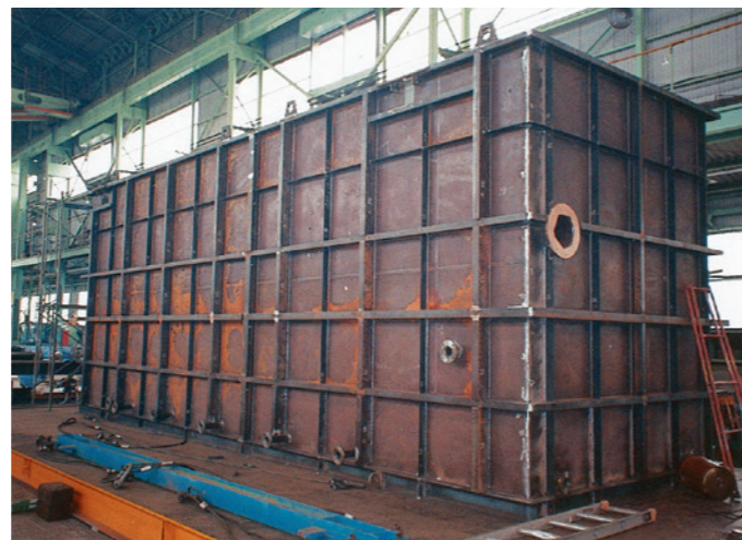
加圧浮上槽 [8,500 L ×2,800 W ×3,450 H ]
